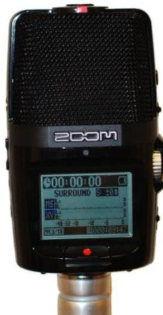
Figure 3.1: Zoom H2N four channel surround sound microphone mounted on a tripod.
