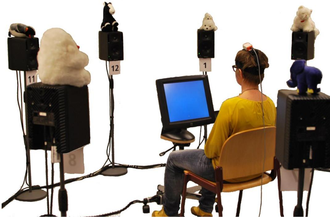
Figure 4.5: Experimental setup in ORL-LEA Room 7 with loudspeakers, feedback monitor and head tracker.
