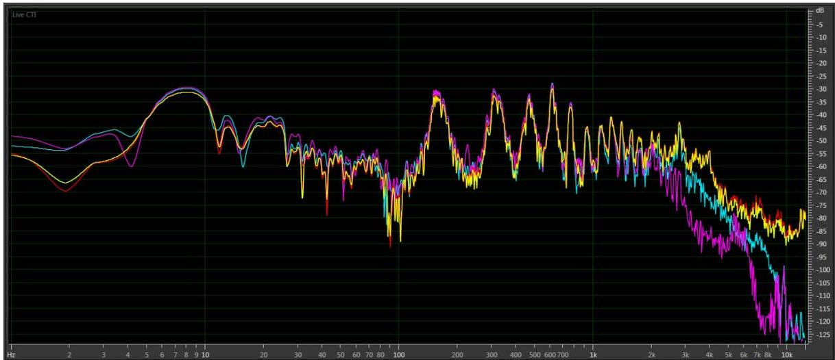
**Figure 110: Frequency analysis of the enhanced signals in comparison to the clean speech signal, when the input is clean speech. Red: clean speech signal. Yellow: enhanced signal with DL. Cyan: enhanced signal with DLW. Pink: enhanced signal with DLW\_SEP.**
