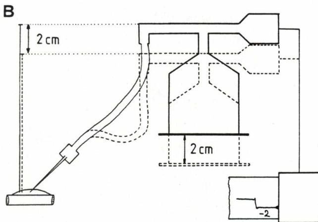
**Figure 1B.** Calibration procedure. Elevating the pump and the pressure transducer on a movable platform 2 cm relative to the pipette results in a pressure increase of 2 cm H<sub>2</sub>O in the pipette on the pump side, which equals a decrease in pressure of 2 cm H<sub>2</sub>O in the fluid under investigation. This pressure decrease is written out on the plotter.
